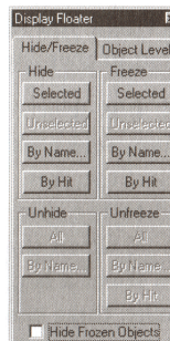
FIGURE 2.15 The Display Floater provides you with modeless access to display commands so you do not need to access the Display command panel.
