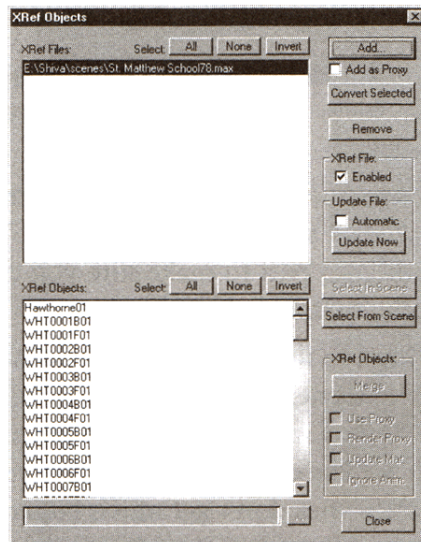
FIGURE 2.5 The XRef Objects dialog box. Here, you can select a scene and any objects in that scene to be referenced into the current scene. You can also use this dialog box to manage those references.
