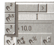
FIGURE 2.26 The snap toggle buttons for MAX. Snaps are not enabled until you enable one or more of the snap toggle buttons.
